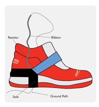
To get the most out of an anti-static floor finish, anyone walking across its surface should be wearing special electro-static dissipative shoes. Without these specialised shoes, the static charge cannot be reliably grounded.
