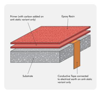
Next, the charge hits a conductive primer that has been filled with carbon to ensure a very low level of resistance. Finally, the charge then hits a copper tape buried under the floor coating which is connected to a safe earthing point.
