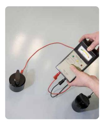
that any charge held by a person is transferred into the floor.
